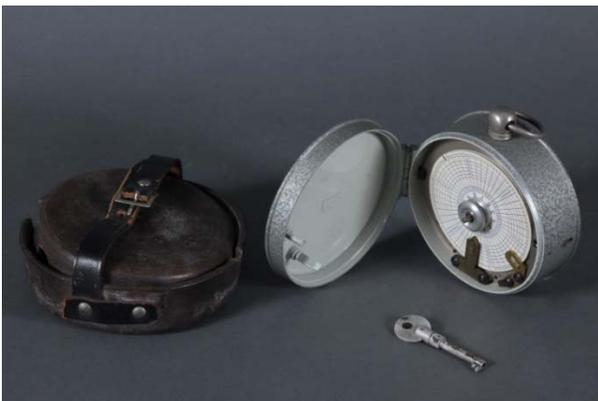
This was used to make sure that the inspection round had been carried out correctly. At different points along the way, there was a key attached to a chain that, when inserted into the clock and turned, marked on a paper disc or ribbon the number of the office and the time. A special device on the cover indicated if the clock had been opened without authorisation, thereby ensuring that the time could not be manipulated.
