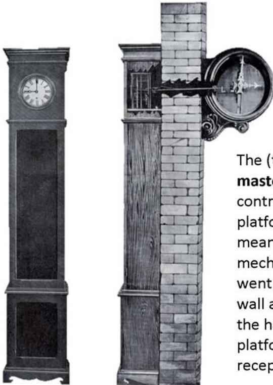
The (tall-case) **master clock** controlled the platform clock by means of a rigid mechanism, which went through the wall and activated the hands of the platform or receptor clock.
